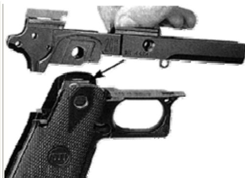
The stud toward the front of the metal upper frame aligns with the hole in the grip frame's trigger guard, and it is secured by a two-headed pin: in the rear, steel plates set into the grip (see arrow) fit into recesses in the frame.
