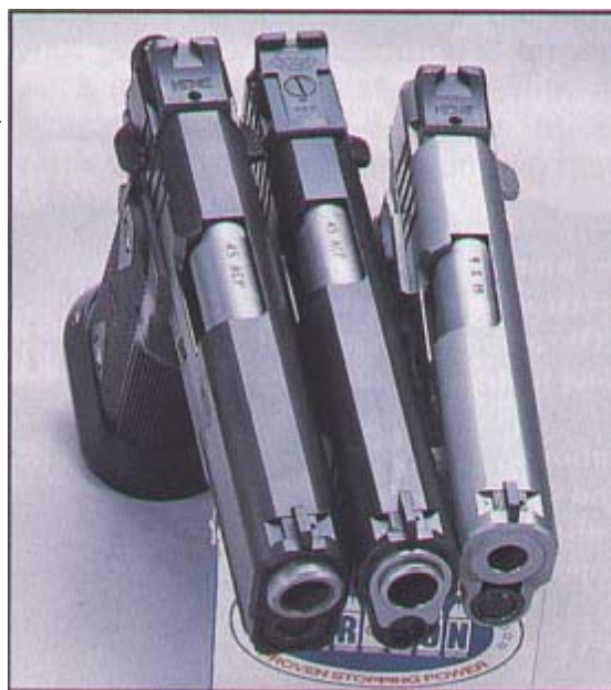
STI guns offer Heinie or STI adjustable rear sights, cone barrel or traditional barrel and bushing.
