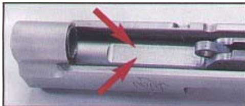
To allow room for the dual spring system, a flat has been milled on the barrel.
