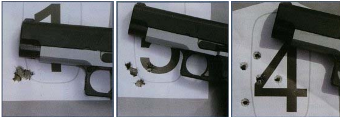
The VIP proved to be exceptionally accurate with handheld groups, left to right, fired at seven, 15 and 25 yards.
