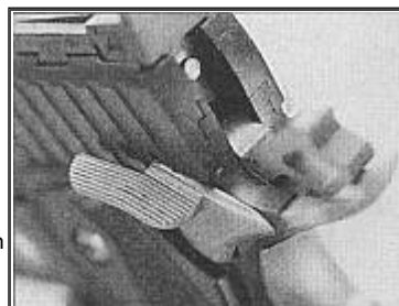
The Competition influence is seen on these STI pistols with the width of the "gas pedal" manual safety lever.
