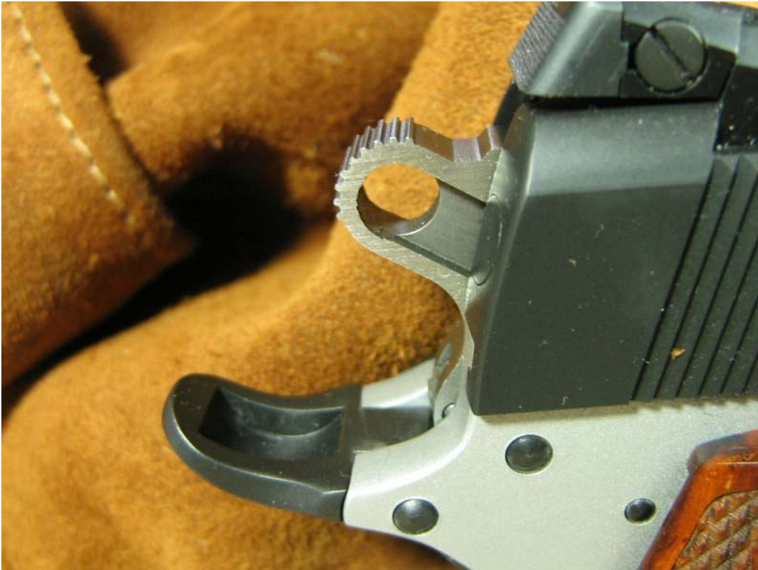
The STI Commander Hammer, high ride beavertail grip safety, and blue pins are visible in this photograph.
