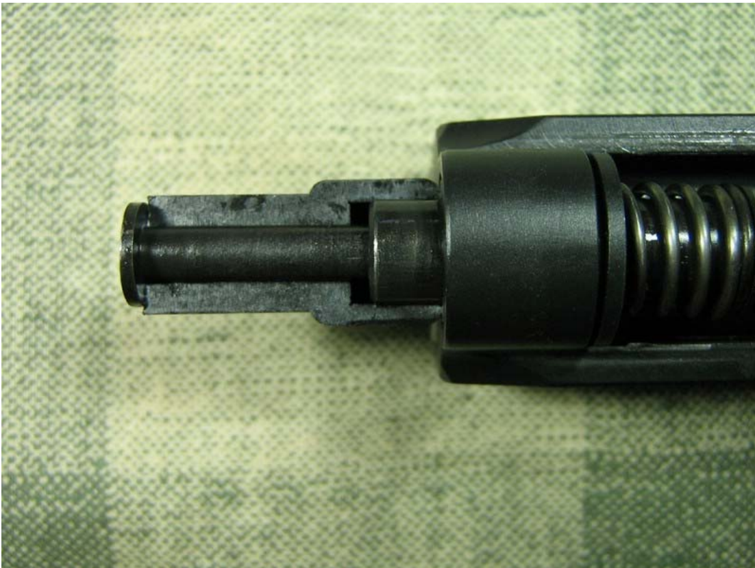
The Take Down tool installed on the Recoil Master guide rod and spring assembly.
