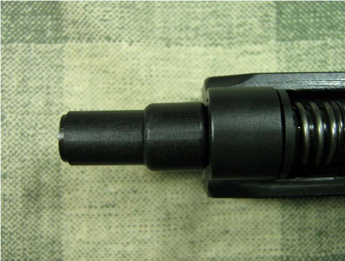
This photo shows (in reverse) how the Take Down tool fits over the Recoil Master guide rod. The Take Down tool must be in this position in order for the Recoil Master guide rod to be removed from the slide.
