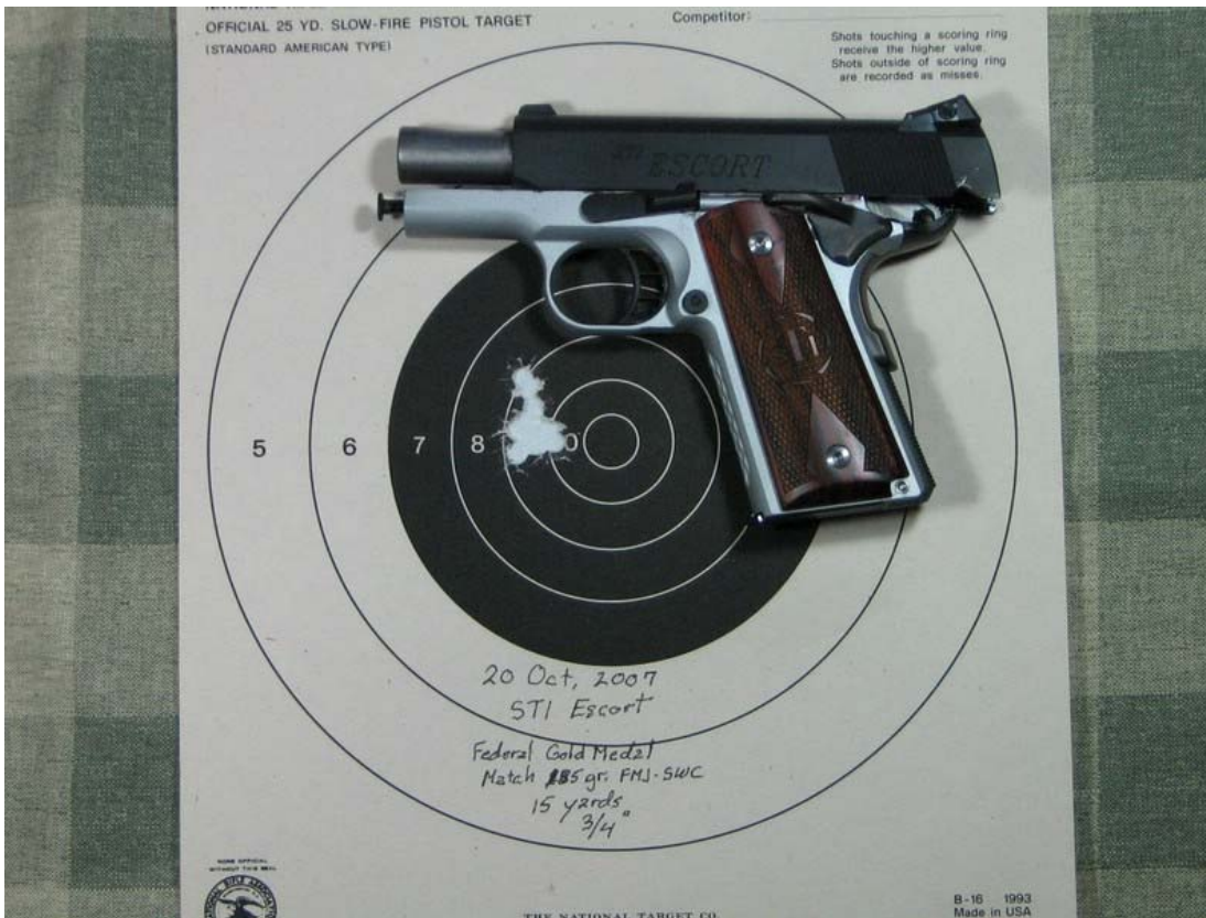
This target was engaged from a distance of 15 yards (45 feet) from the muzzle of the STI Escort. The vertical spread measured seven-eighths of an inch. Ammunition was Federal Gold Medal Match 185 gr. Full Metal Jacket/Semi-Wad cutter.
