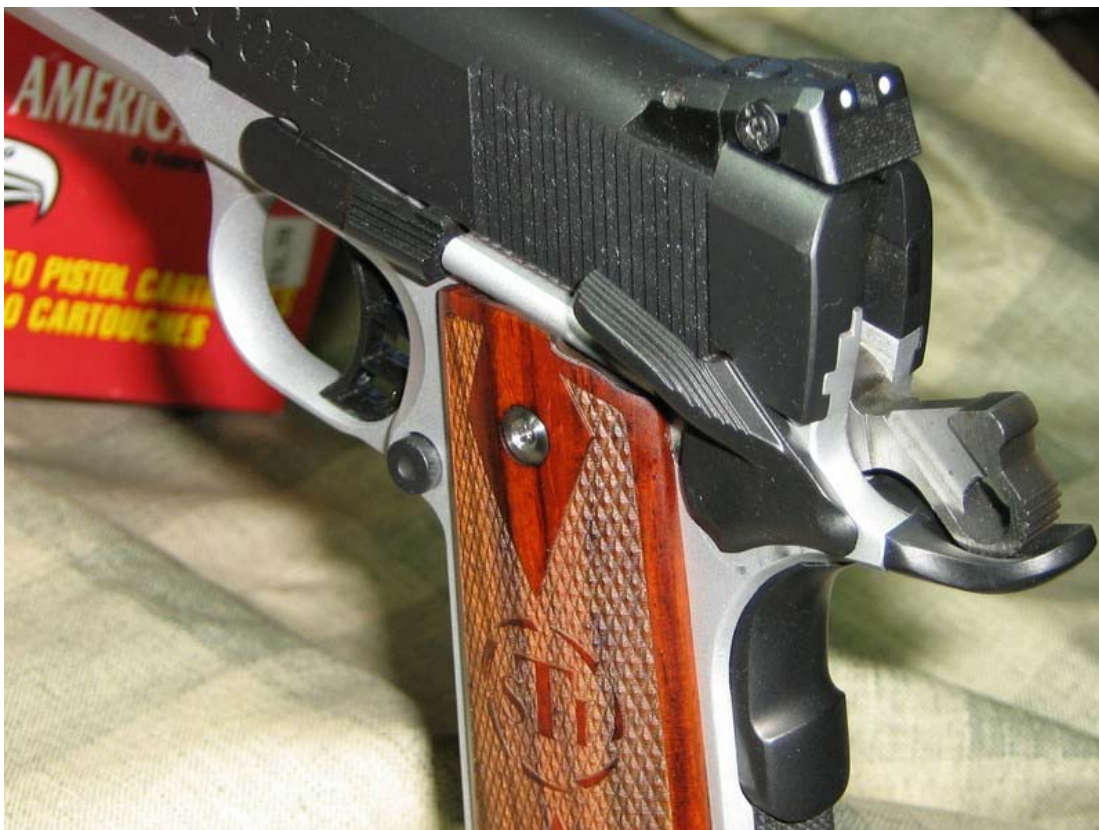
A side view of the T.A.S. sight, as well as the cocking serrations and the single extended shelf thumb safety, are displayed in this photograph. The beavertail grip safety is also shown in this photo.
