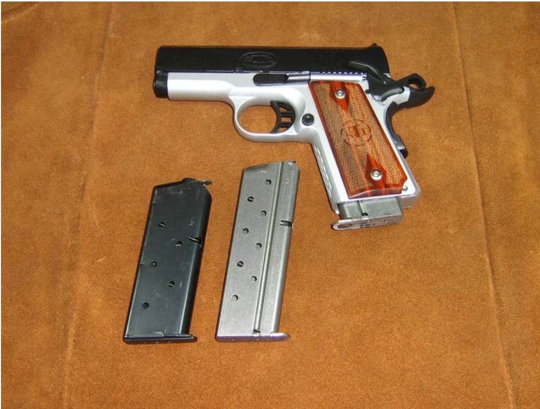
This photograph illustrates the difference in the size between the STI Rogue and standard Officer sized pistols. The Metalform "Springfield" 9mm magazine hangs 3/8" from the bottom of the pistol when locked in place. The issued Metalform magazine is pictured on the left, with the "Springfield" magazine from Brownells on the right.
