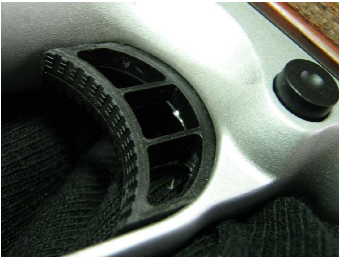
The STI Long Curved Trigger and smooth magazine release are featured in this photograph. The trigger face is a glass filled nylon polymer with over travel adjustment screw. Twenty repetitions with a Lyman Digital Trigger Pull Gauge yielded an average sear release at 4 lbs. 15 ounces (260gms.). Approximately 3mm of take-up led to a crisp release.
