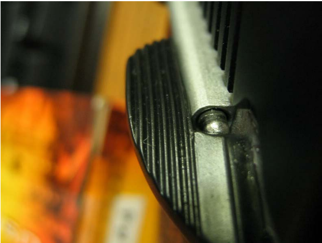
The extended single-side thumb safety is perfectly matched to the plunger pin and housing.
