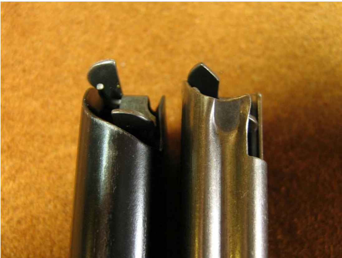
This photograph illustrates the difference in the size between the STI Rogue and standard Officer sized pistols. The Metalform "Springfield" 9mm magazine hangs 3/8" from the bottom of the pistol when locked in place. The issued Metalform magazine is pictured on the left, with the "Springfield" magazine from Brownells on the right.
