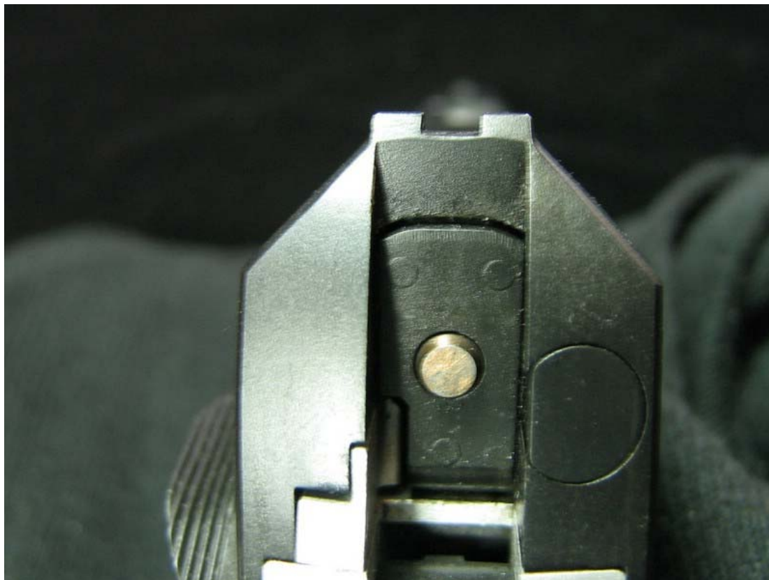
This view, from the rear of the slide, shows the integral rear sight, the back of the ejector, and the fine fitting present on this end of the pistol.
