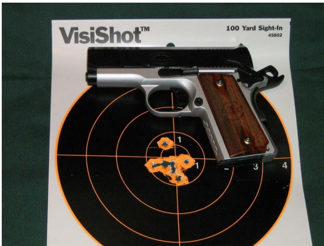
This photograph depicts the results of eight shots fired from a distance of 25 feet using a standing two-handed hold on the STI Rogue. Ammunition is Remington UMC 124 gr. Full Metal Jacket.
