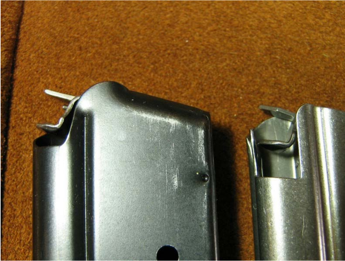
These two photographs show the differences between the issued Metalform magazine's follower and the follower of the Metalform "Springfield" magazine.
