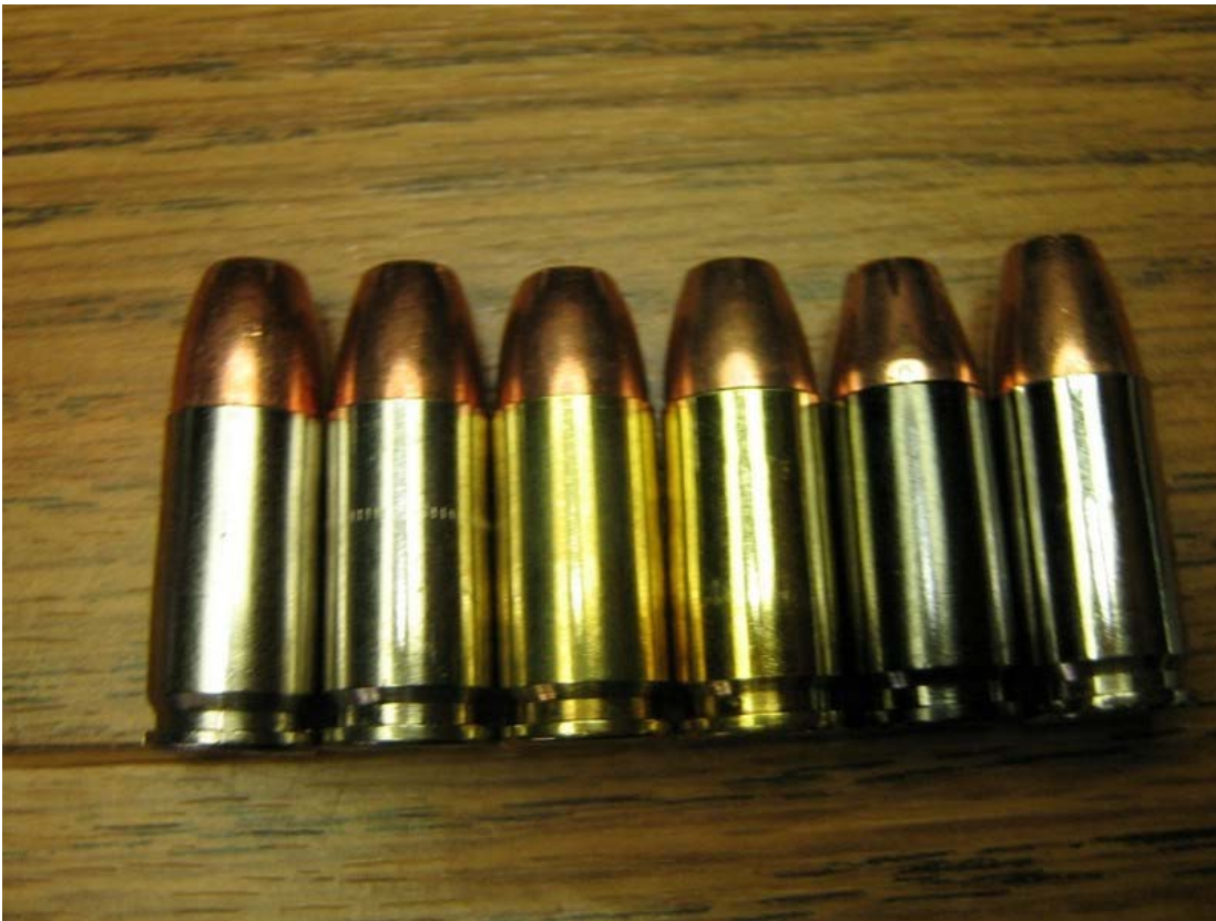
Jacketed Hollow Points and Truncated Cone Hollow Points used in the testing of the STI Rogue.
