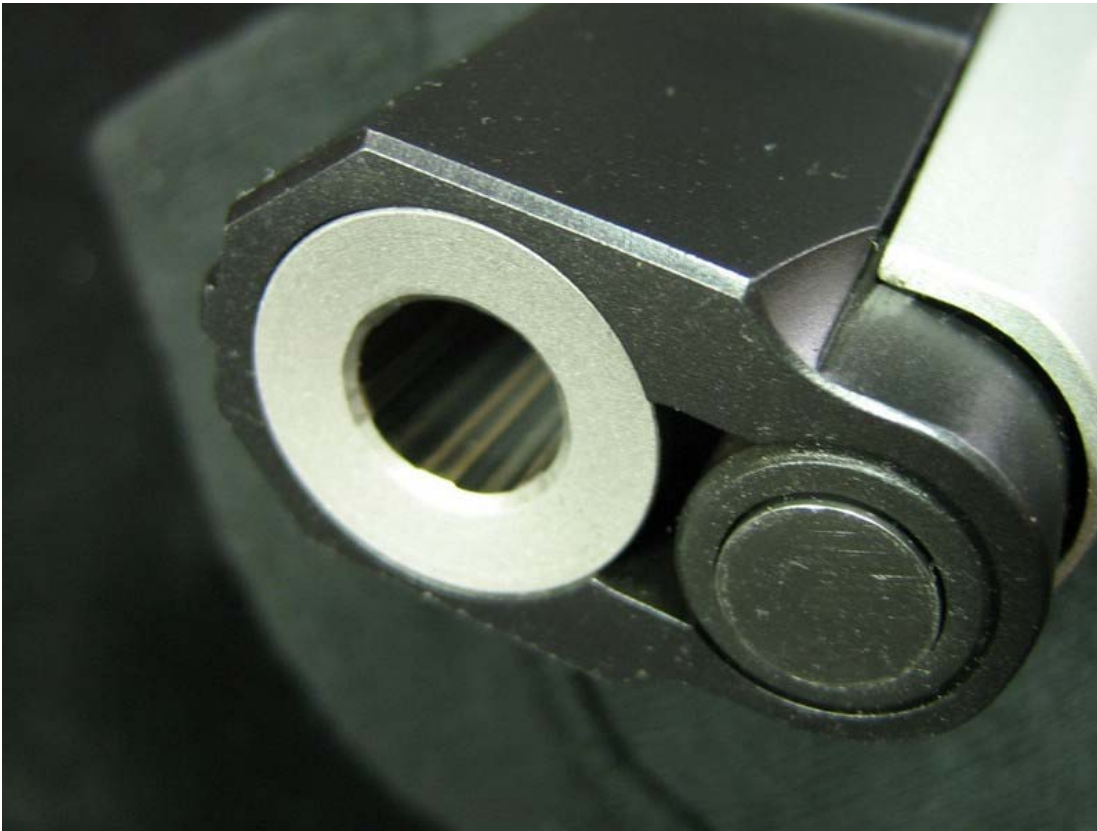
Photograph taken from the muzzle end of the pistol, showing the beveled modified cone barrel and end of the Recoil Master Guide Rod assembly.
